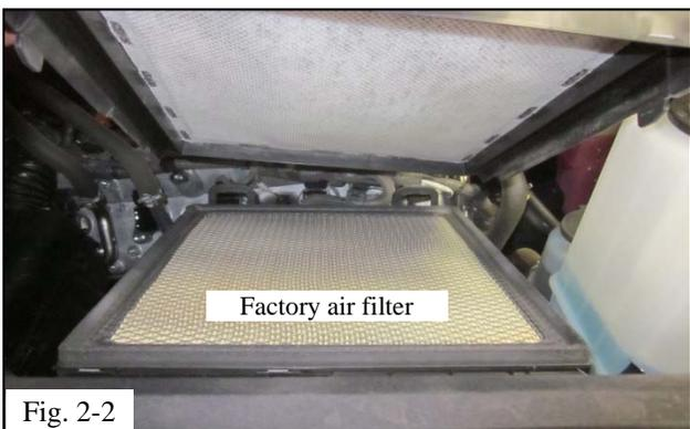
**3. Install the TRD Air Filter.**
